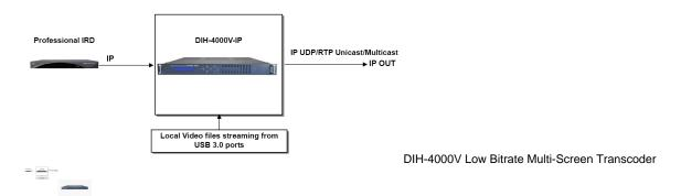
The DIH-4000V low bitrate H.264 Real Time Transcoder is specially designed for IPTV system, especially for those IPTV systems over unmanaged network architectures in which the bandwidth are normally limited. Adopting the powerful chip sets and high efficient SD/HD decode/compression algorithm, the inputted programs (Video + Audio) can be transcoded (re-compressed) into relative low bit rate (
